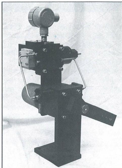
**R**EXA Xpac drives feature a self contained Electraulic power module utilizing the patented Flow Match System. This technology allows precise positioning independent of load variation and locks the cylinder in place when no movement is required. Hydraulic flow is generated by an internal positive displacement gear pump driven by a continuous duty motor without limitations on start, stop, or reverse cycles.
