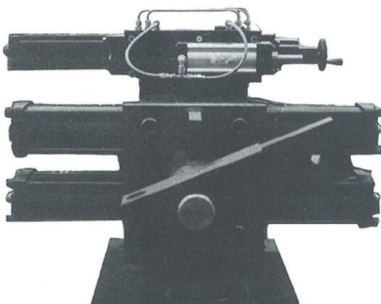
The D series drive is designed by combining the R Series actuator and a drive mounting base. Torques from 600 in-lbs to 100,000 in-lbs are standard. The base is attached to a user prepared pad by a 4 bolt pattern. A drive arm is custom designed to meet a particular installation.
